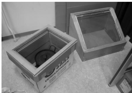
Two different models of the Solar Box made with cardboard, paper and pap glue (Paper-based Technology) by Marjan Velthuijs and Henk Blok.
