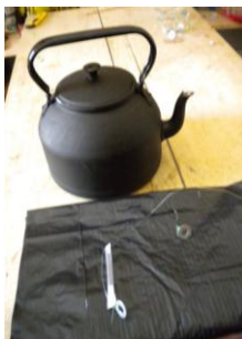
Water Pasteurisation Indicator (WAPI)
