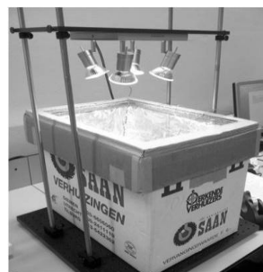
Two different models of the Solar Box made with cardboard, paper and pap glue (Paper-based Technology) by Marjan Velthuijs and Henk Blok.
