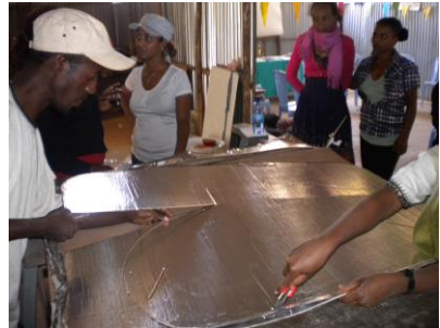
Let the foil dry thoroughly, then cut the CookKit with a template
