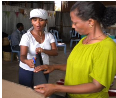
Cut strips of fabric to glue around the edges to protect the CookKit
