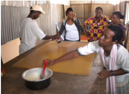
First apply glue on cardboard, then rub foil onto cardboard
