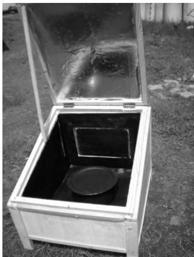
Improved Solar Box, for a 5-litre pan with a small door at the back to open the box. Design Bereket Dessie, Addis Ababa.
